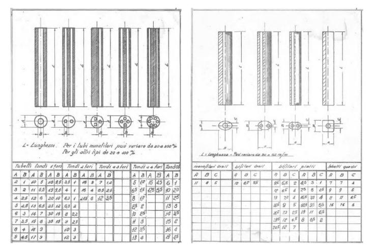
External diameter of tubes can reach up to 70mm with a length of 600mm also as function of the thickness
